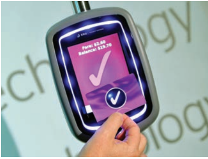
FIGURE 3.34 The myki public transportation ticketing system uses near field communication to read a commuter's details from their smart card.
