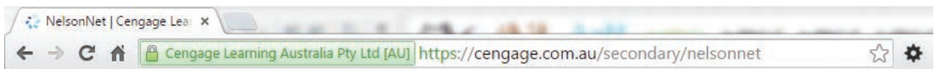
FIGURE 3.18 A secure connection is indicated by 'https://' appearing in the URL and the lock symbol, in this case to the left of the address bar.
