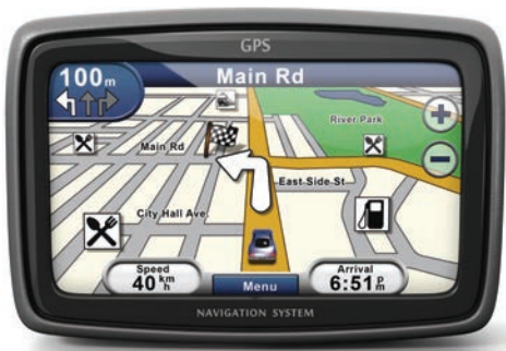
FIGURE 3.23 The GPS navigation device receives three-dimensional data from a satellite network, which enables the receiver to pinpoint the car's location and give travel directions to the driver.
