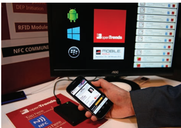
FIGURE 3.33 An example of a near field communication use for short-range contactless communication.
