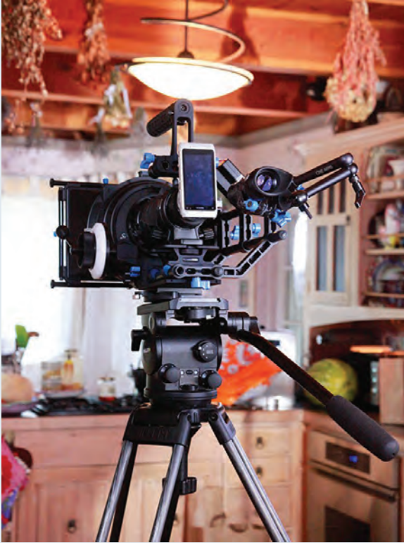
Figure 17.36 One of the camera rigs for Olive (2011), assembled by the team after they deconstructed a 1940s film camera to solve the technical challenges themselves. Among the solutions was a final touch of attaching the phone with double-sided tape – a surprisingly basic solution for a film that cost just under half a million dollars to make.
