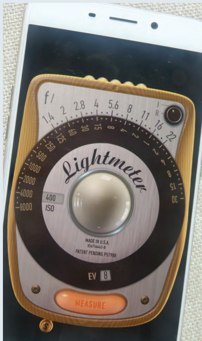
Figure 17.15 Traditionally, light meters were analogue devices. Nowadays, light meter apps are available for smartphones to help judge the contributing intensity of each light.
