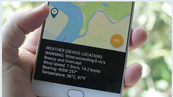
Figure 5.22 CASA’s drone safety phone app Can I Fly There? is designed for drones under 2 kilograms (excluded category), and is useful on location. It has built-in weather warnings and shows current permissions.
