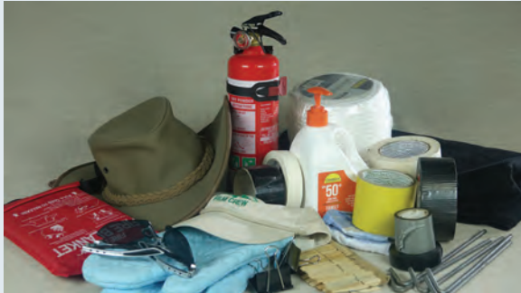
Figure 5.29 Among items to have on hand at a set is gaffer tape (waterproof cloth tape). Named after the film job, gaffer tape is used to secure cables on music and theatre stages. Sound crews need to tape audio cables separately, crossing power cables at 90 degrees to reduce the buzz created by induced current in the audio trip hazard cables. Tape is also used for ‘marks’ on the floor for actors, and camera tape has a particular meaning for the crew depending on the colour and where it is applied, such as a film can or magazine.
