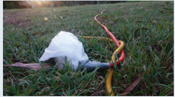
Figure 5.33 Electrical cables should not be on the ground near water or rain. Dew can even get into extension cable joins on an early morning shoot. Plastic bags reduce moist air in the cable ends, and a loose knot helps prevent cables detaching. Adult supervision would be expected for using electricity, and a cable on the ground of a public footpath is one of the triggers for some councils to require a filming permit.
