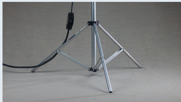
Figure 5.31 Lighting stands should be arranged to create the broadest base possible, and secondary safety chains must be used when rigging lights to a properly installed and rated studio ceiling grid.
