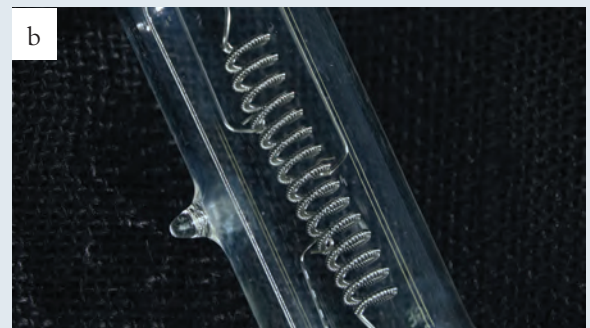
Figure 5.34 Filament bulb lights will blow if moved when hot, or if the bulbs are touched by the oil on human skin. Let them cool before packing up so the tungsten is less fragile.
